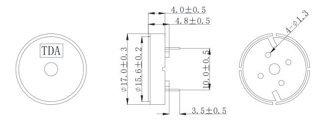
Unit:mm Tolerance: ±0.5mm
